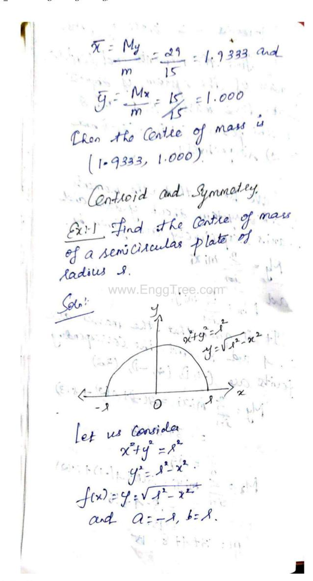
there there is no need to use the formula to Calculate  $\bar{\chi}$ , because, by the symmetry principle, the Centre of mass must lie on the y-axis. Hence  $\bar{\chi} = 0$ . the Area of the semicicle is A= 1, 1112 Now y = 1/A (f(x)) dx. 7 =0, 4=4/3/h
